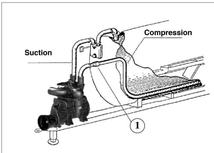
The Rotary blades vacuum pump can be used as a mixer by fitting, on request, a double outlet on the manifold (see Figure 2). In this case there will be the intake of a normal Rotary blades vacuum pump, but a perforated tube placed inside the tank car must be used for the compression.
